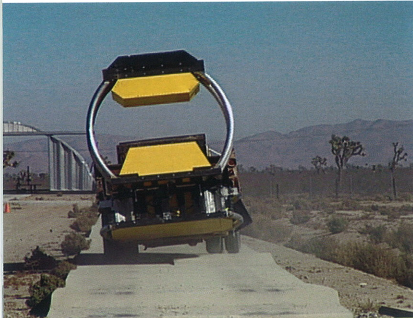
The Scorpion TMA, being driven over a variety of curbs, bumps, risers and drop-offs.
