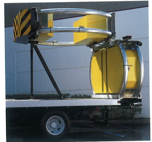
Flat-bed truck with Center Post Bracket.
