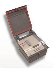
The Peek ADR-2000 Plus can be used as a portable or semi-permanent unit. In its basic configuration as a counter/classifier, 2 or 4 road tubes are available. With optional internal sensor modules, the ADR-2000 Plus can monitor up to 42 inputs using a combination of WIM, loops, piezos or contact inputs.
